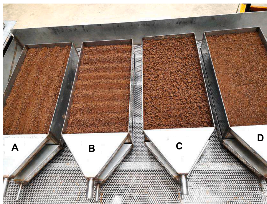
Fig. 1. Four roughness treatments applied to a sandy loam soil in erosion trays: oriented roughness – up/downslope direction (A), oriented roughness – across slope direction (B), random roughness – non directional (C), and smooth surface – with no roughness treatment applied (D).
