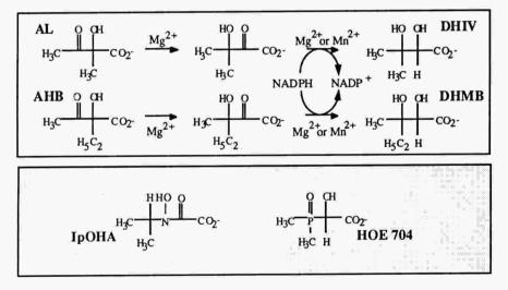
Figure 1: Reactions catalysed by KARI and the structure of IpOHA and HOE 704. Abbreviations: AL, 2-acetolactate; AHB: 2-aceto-2-hydroxy butyrate; DHIV, 2,3-dihydroxy-3-isovalerate; DHMV, 2,3-dihydroxy-3-methylbutyrate.
