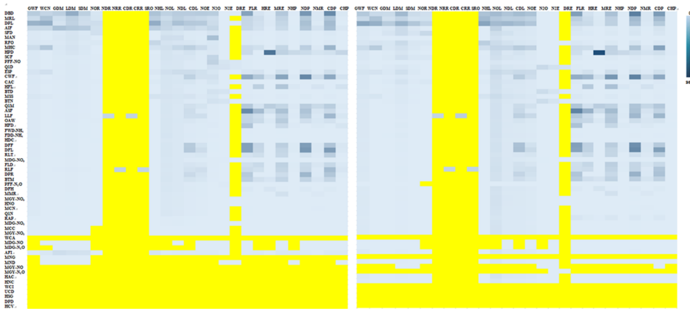
Figure 3. Heat maps of averaged NRMSDs for the 61 parameters (rows) with respect to the 27 output variables (columns) with the climate condition in South West England from individual years (left) and the pairs of consecutive years. (right). A yellow pixel represents no interaction.
