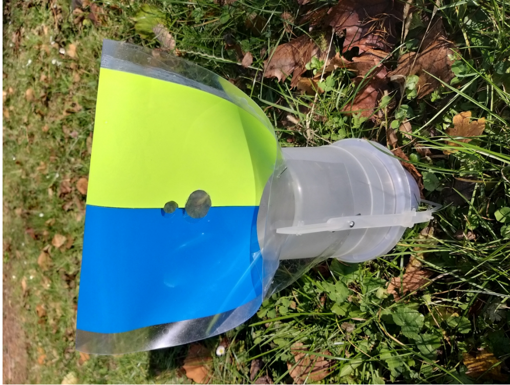
Fig. 2. CSALOMON® VARb3 funnel trap used in Exp. 3. One half of the upper panel of these traps was fluorescent yellow and the other half blue.
