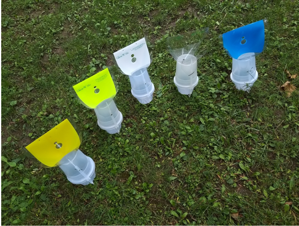
Fig. 1. CSALOMON® VARb3 funnel traps (Plant Protection Institute, ARC ELKH, Budapest, Hungary) used in field trials. The upper panels of the traps were (from left to right) yellow, fluorescent yellow, white, transparent and blue.
