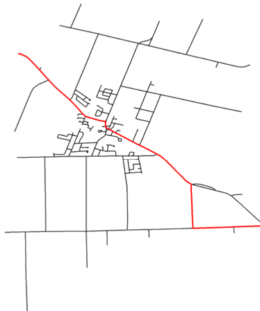
Figure 15. Finding the network diameter with shp2graph and igraph (Ontario road data).
