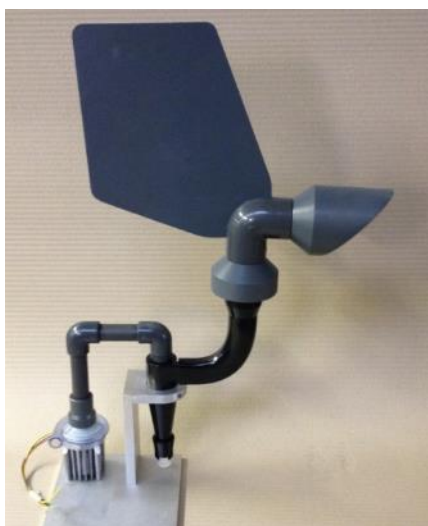
Figure 2. Compact, high volume cyclone with rotating air intake, sampling at 300 L/min with excellent collection efficiency of particles down to at least 4 \mu\text{m} aerodynamic diameter.
