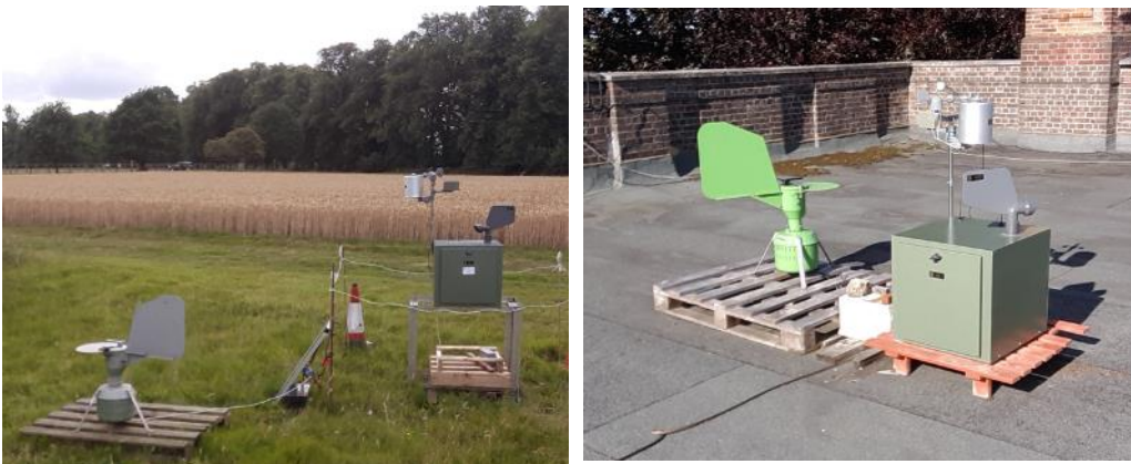
Figure 10. Automated spore traps operating at two locations at Rothamsted in summer 2017 next to seven-day spore traps.
