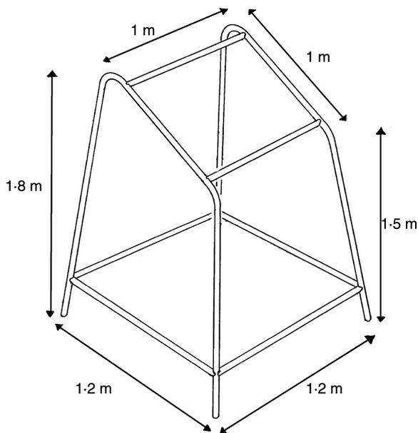
Figure 2 The basic aluminium frame of the tent manufactured from 2.5 cm diameter tubing.
