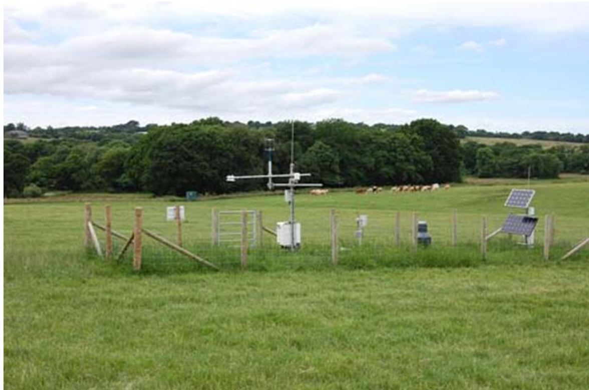
Figure 17. COSMOS-UK Soil moisture monitoring equipment on Catchment 2.
