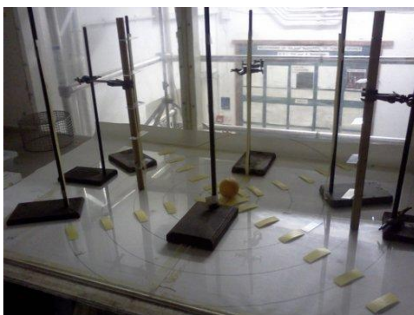
Figure 6: Rain splash experiment at the base of the 11 m Rothamsted Rain Tower; water sensitive paper strips placed vertically and horizontally at various distances and heights from target orange
