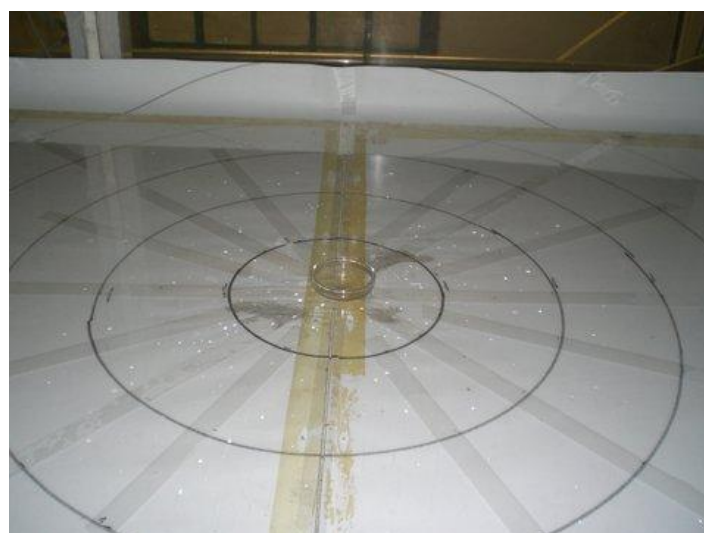
Figure 10: Splash collection at base of rain tower on melinex strips
