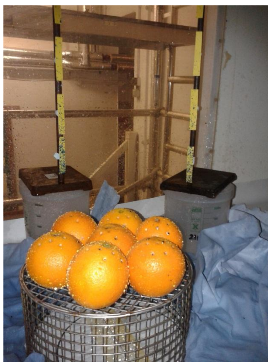
Figure 7: Multiple rain splash experiment in Rothamsted Rain Tower; batch of infected oranges on metal cage and surrounded by tissue to soak up excess splashes P. citricarpa spore suspension
