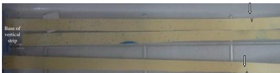
Figure 16: Splash pattern on vertical strips of water sensitive paper; the splashes are more dense at the base of the strips (left hand side of figure) and less frequent at the top. The height of the maximum splash is marked by an arrow.
