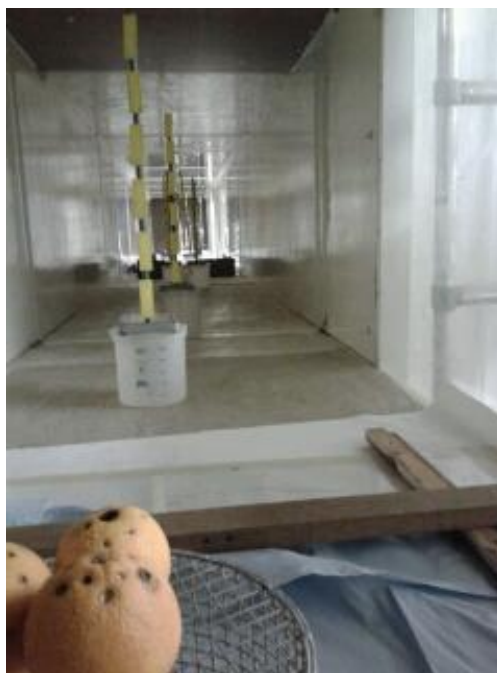
Figure 8: Rain splash and wind effects experiment in the combined Rothamsted Rain Tower-Wind Tunnel facility; rods with water sensitive paper strips placed downwind from the infected oranges up to a maximum distance of 8m
