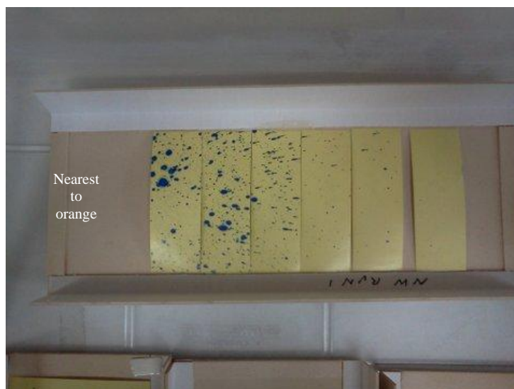
Figure 19: Splash pattern on horizontal strips of water sensitive paper; the splashes are clearly more dense on the strips nearer the orange (left hand side of figure) and less dense further away from the orange (note: wsp strips shown rearranged to be closer together than in the experiment).
