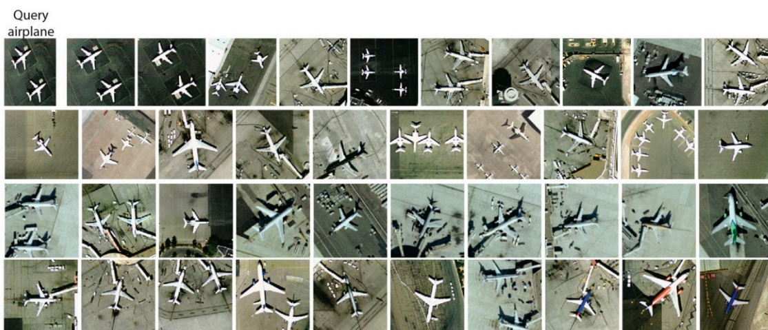
Figure 10. Retrieval results of airplane category using convolutional neural network as a feature extractor (RL-CNN). The methods obtained 100% retrieval accuracy.
