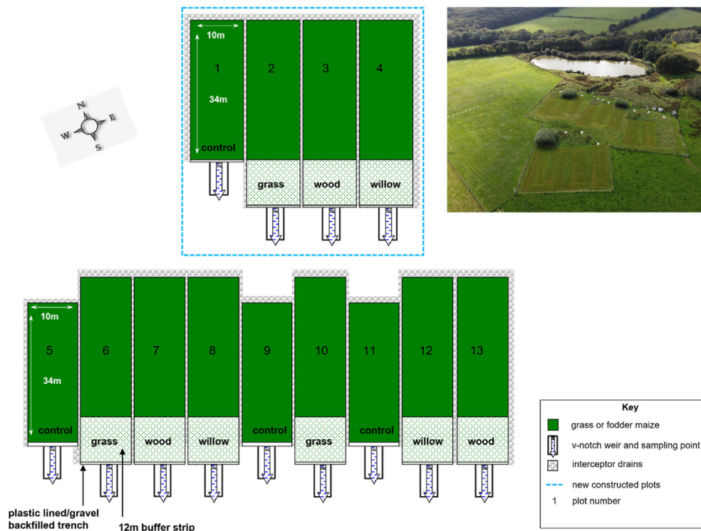
FIGURE 1 Schematic of the experimental platform and aerial photograph of the experimental facility, showing the replicated buffer plots.
