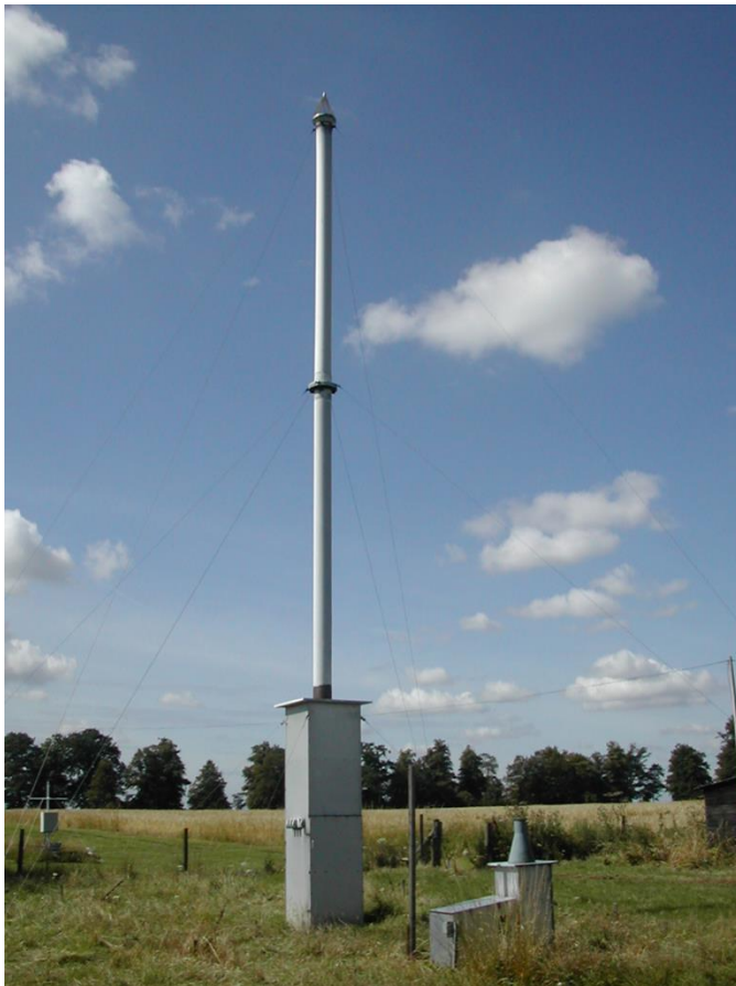
Fig. 1. The Rothamsted Insect Survey's 12.2 m suction-trap used to sample aphids.
