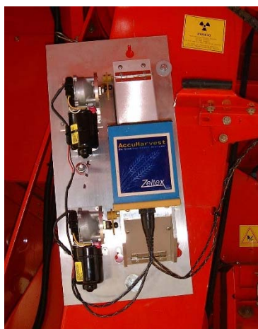
Figure 67. Zeltex AccuHarvest protein sensor mounted on grain elevator
