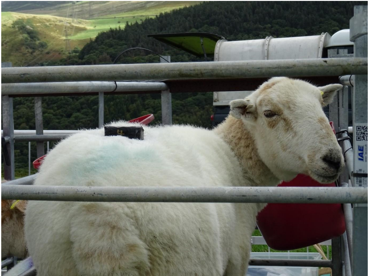
648 Fig. 1. Daily Diary sensor (accelerometer) glued to the hind of a Welsh Mountain 649 ewe.
