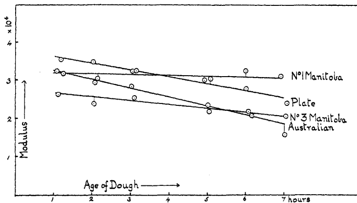
FIG. 4. The effect of age of the dough on the modulus
