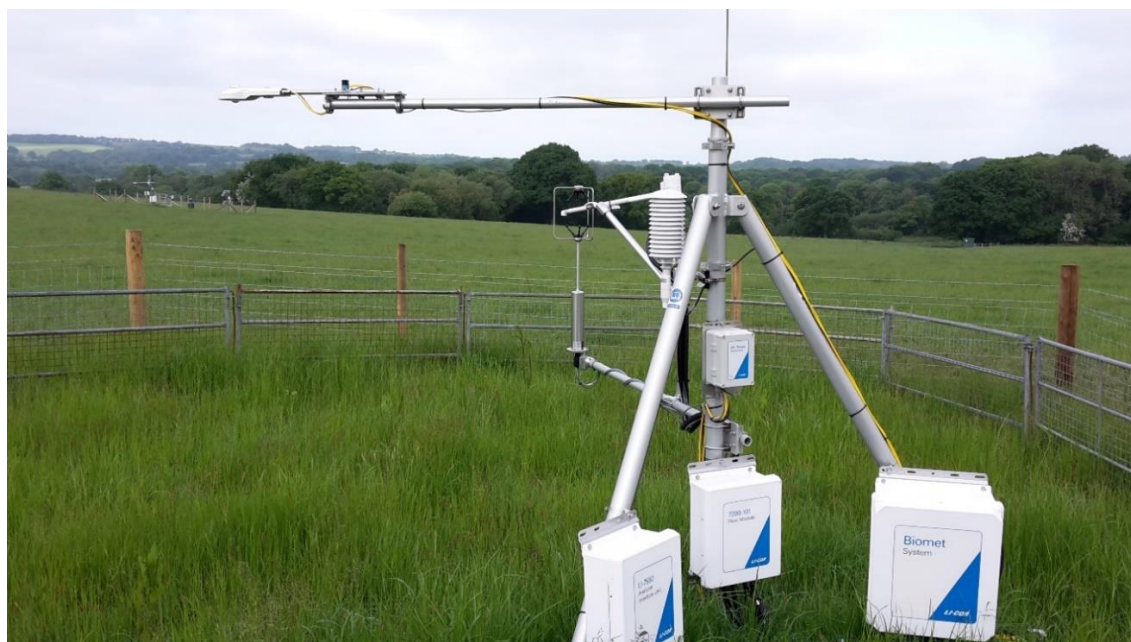
Figure 3. Eddy Covariance tower and monitoring equipment.
