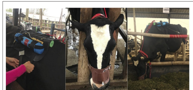
FIGURE 1 | Cow equipped with the sulfur hexafluoride (SF 6 ) equipment to measure enteric methane (CH 4 ) emissions. From left to right: the saddle with PVC canisters; leader head halter, with the sampling point; and the entire equipment.
