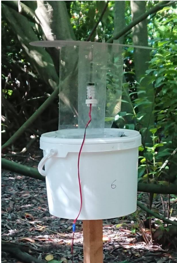
Fig. 3.3. UV LED moth-trap (live-trap – prototype v.1.1).
