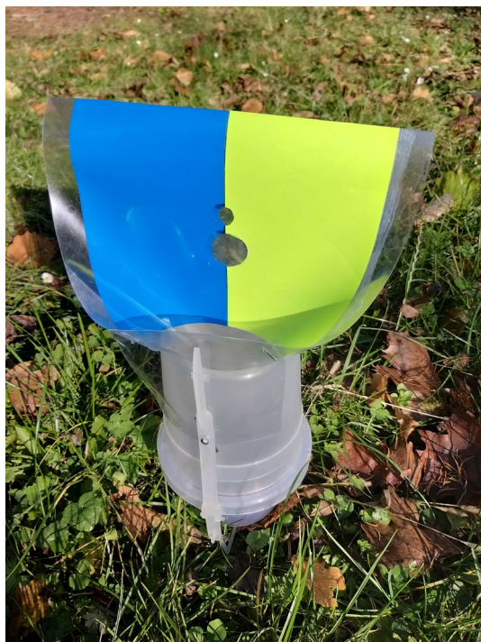
FIGURE 2 CSALOMON® VARb3 funnel trap used in Experiment 3. One half of the upper panel of these traps was fluorescent yellow and the other half blue
