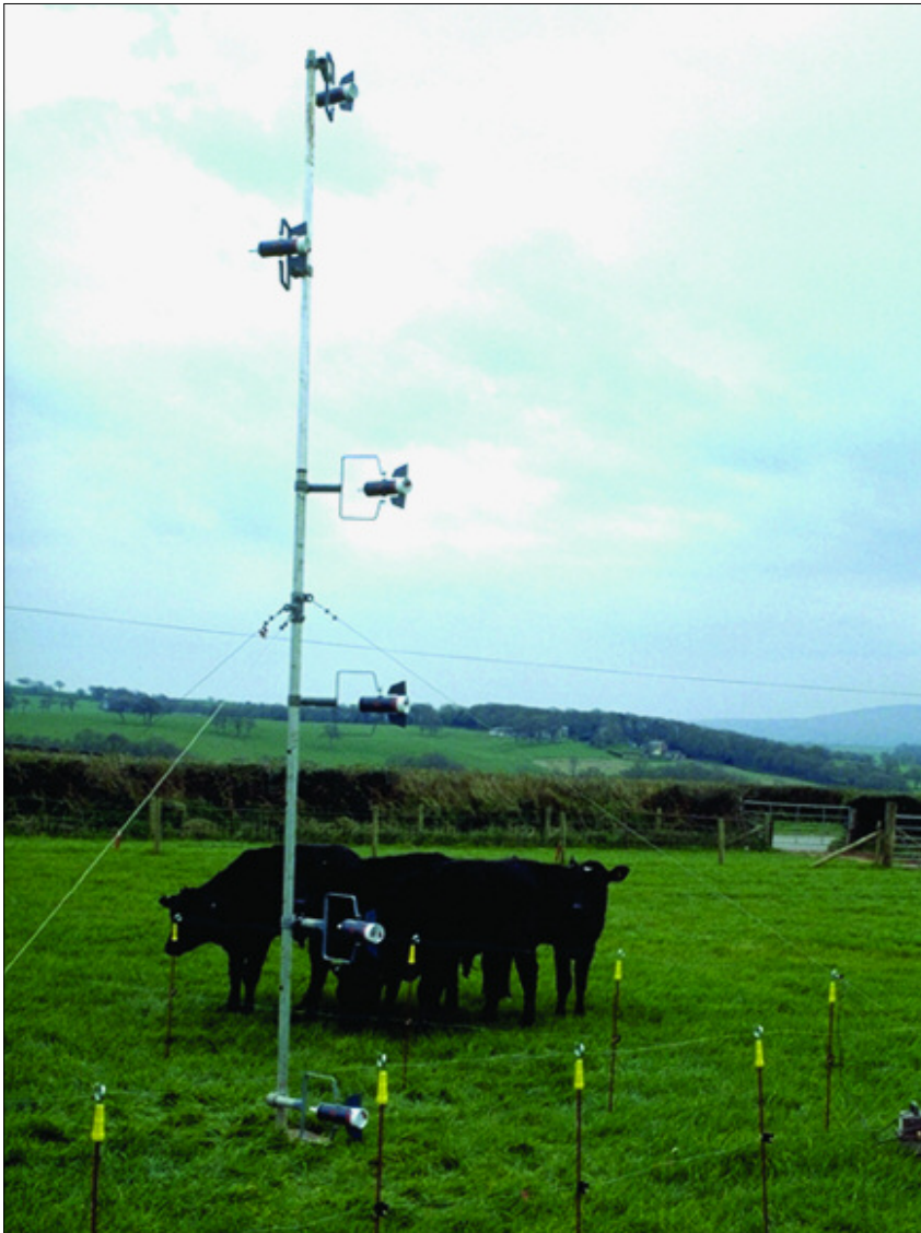
Figure 7.1 Measuring ammonia volatilisation from grazing livestock
