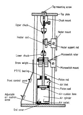
Vertical adjustment of the microswitch mounting assembly is made by sliding it on the main support rods and is automatically retained in position by two pre-tensioned nylon screws.
