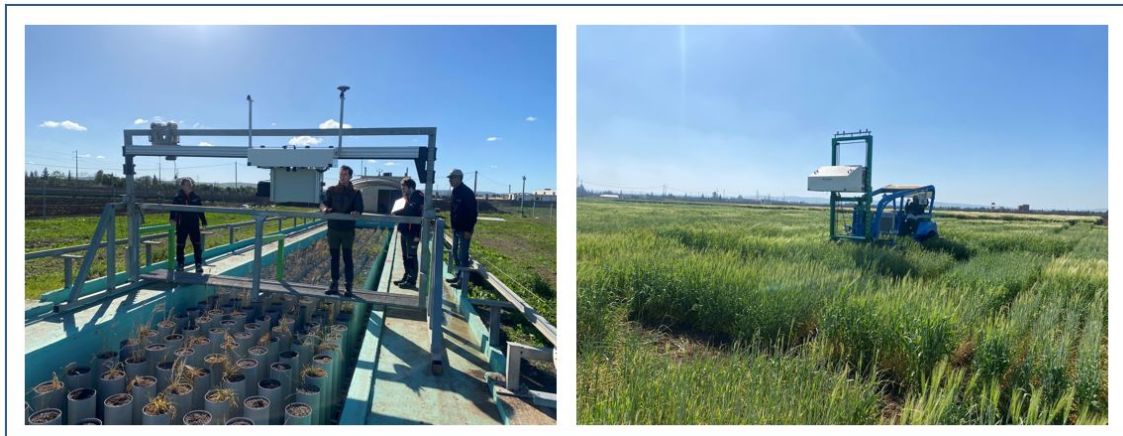
Figure 2.4. The ICARDA's precision field phenotyping platforms installed at Sidi el Aidi (Settat) in Morocco. Images are in courtesy of Andrea Visoni of ICARDA-Morocco.
