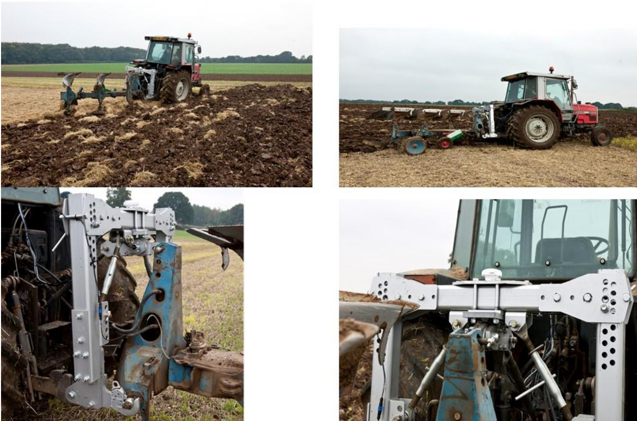
Figure 3.1 Images of the draught sensing frame in place between the tractor and the plough
