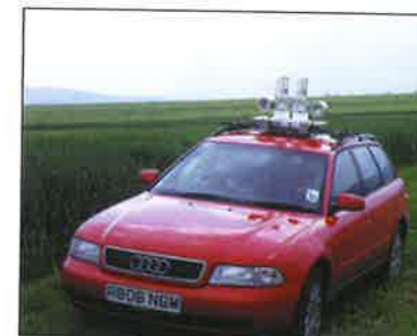
Wind impaction spore trap on a car roof. This is used, especially for Erysiphe graminis , to conduct surveys to monitor the development and status of fungicide resistance (Zeneca)
