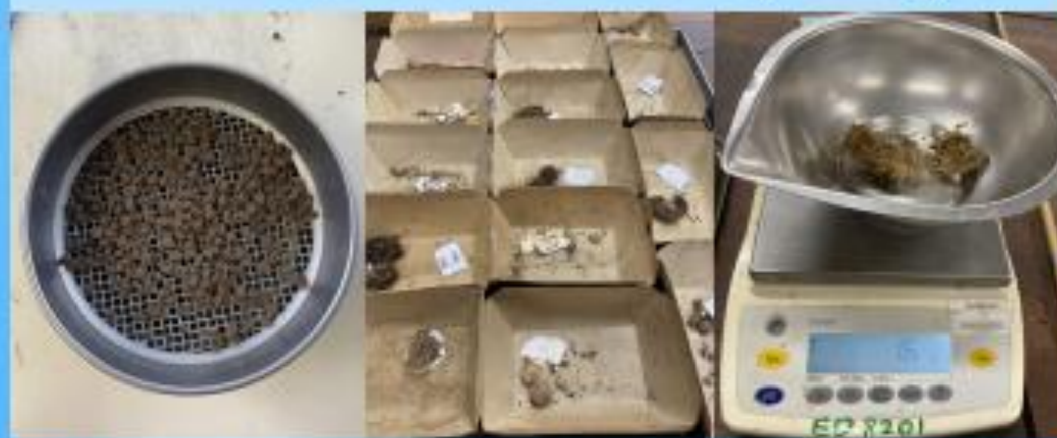
Figure 4: Accounting for stones when measuring bulk density: Sieve dry sample using a 2mm sieve and weigh sample collected in the 2mm sieve - minus this measurement from wet and dry soil weights.
