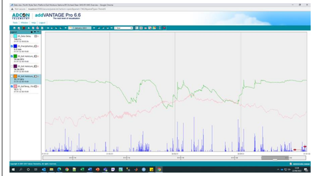
Figure 3. Example of graphical display by the addVantage Pro software of soil moisture, soil temperature and rainfall data for one of the catchments.
