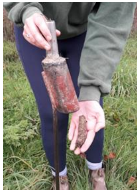
Figure 12. 10 cm deep soil pot corer.
