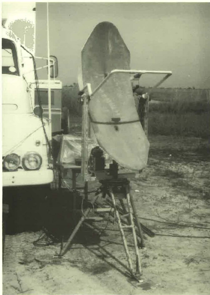
Figure 6 A range height indicator (RHI) radar built by the NRI Radar Unit, and deployed in Mali in November 1974. This radar oscillates or ‘nods’ once every 3 s over a range of 60° in the vertical.
