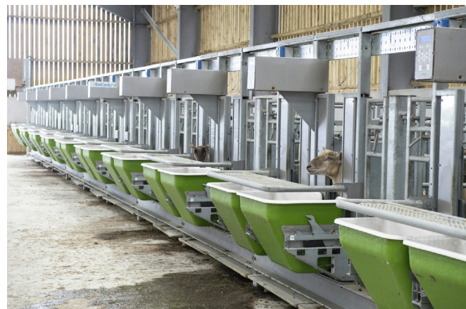
Fig. 1. BioControl CRFI. Sheep were housed within BioControl 'Controlling and Recording Feed Intake' (CRFI) pens throughout the acclimatisation and experimental periods. Animals were allocated to an exclusive Biocontrol feeder (green bin pictured), access to which was granted by vertical sliding feed gates, controlled by animal-specific individual electronic identification ear-tags.
