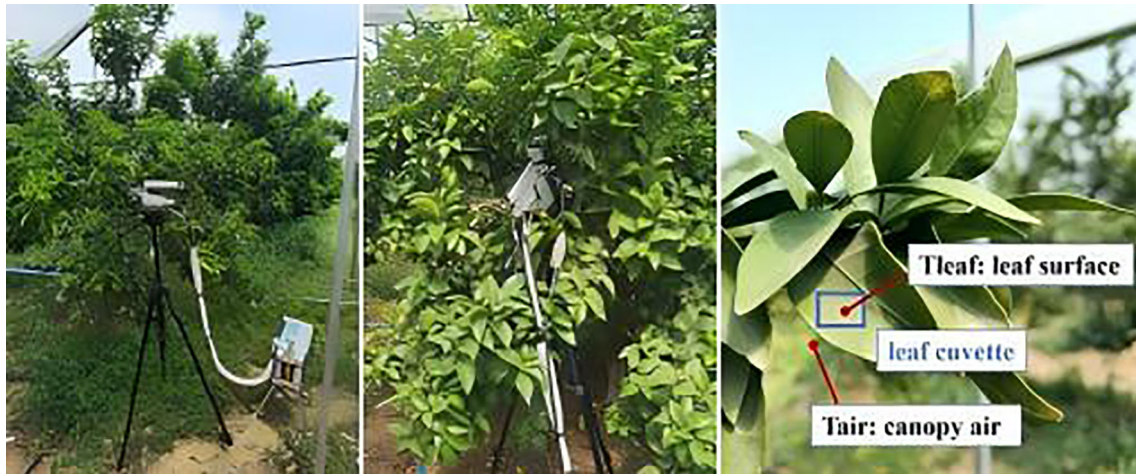
FIGURE 2 Leaf gas exchange measurements using a portable photosynthesis system.
