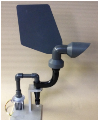
Figure 2. Compact, high volume cyclone with rotating air intake, sampling at 300 L/min with excellent collection efficiency of particles down to at least 4 µm aerodynamic diameter.
