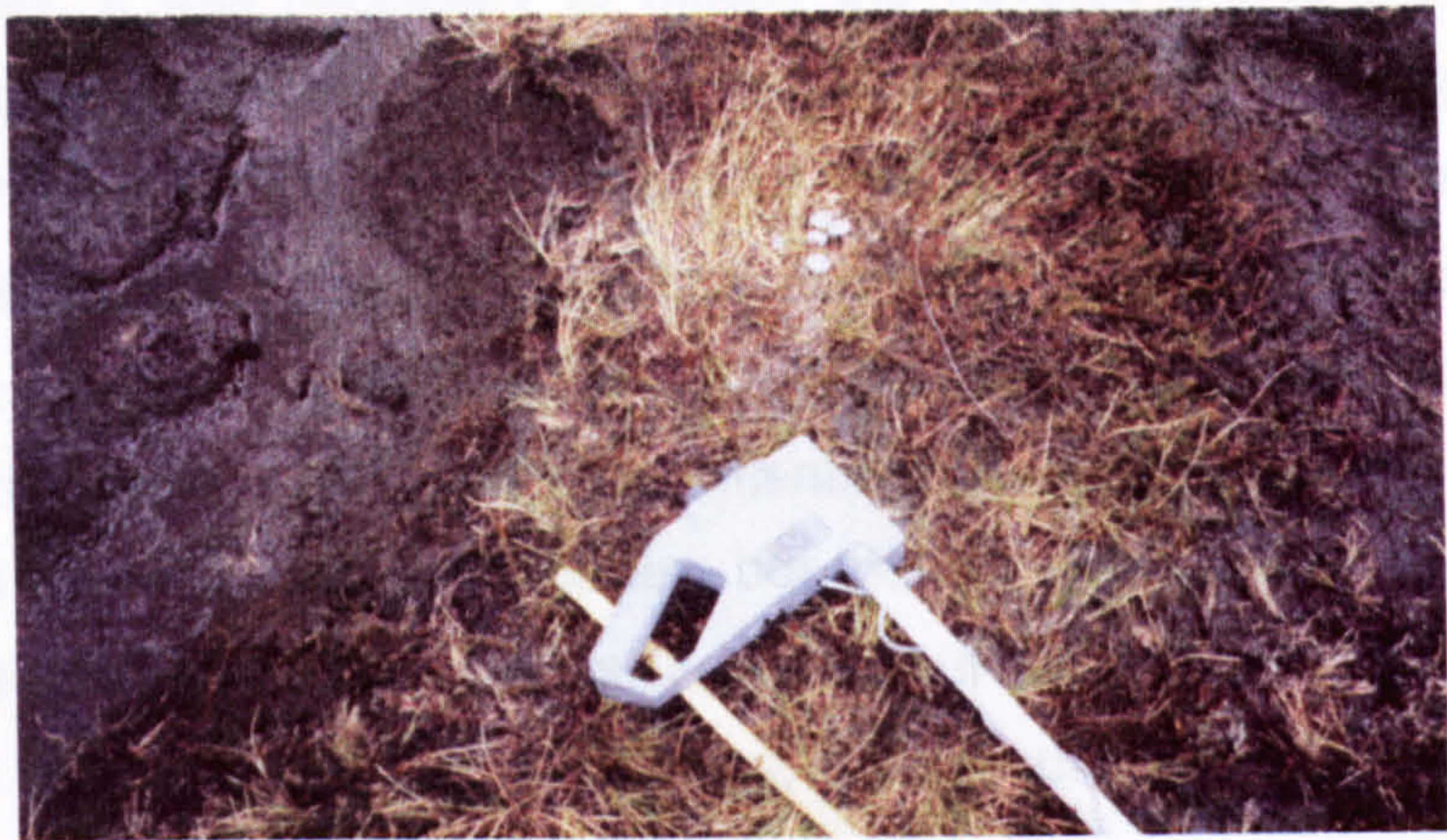
Plate 4.2 Arrangement of nails in ground two years after placement. Part of the metal detector used to relocate nails is also shown (Yorkshire Dales).
