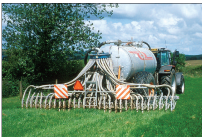
Fig 10.1 Slurry application to the soil surface using trailing shoe equipment
