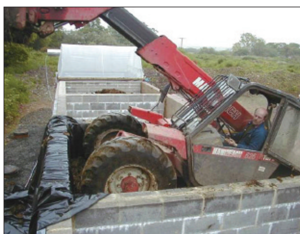
Fig 10.4 Compaction of solid manure heaps to maintain anaerobic conditions
