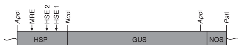
Figure 1 Diagrammatic representation of pHSPdGUS. HSP indicates the 3' end (656 bp) of the Hvhspl7 gene promoter containing the two heat-shock elements and the metal response element identified by Marmiroli et al. (1993). GUS indicates the β-glucuronidase reporter gene. NOS indicates the nopaline synthetase terminator sequence. Target sites for restriction enzymes used in cloning are indicated (note that there are two additional Apo I sites in the vector sequence downstream of the NOS terminator). The plasmid vector is pGEM7zf(-) (Promega UK Ltd., Southampton, Hampshire, UK).
