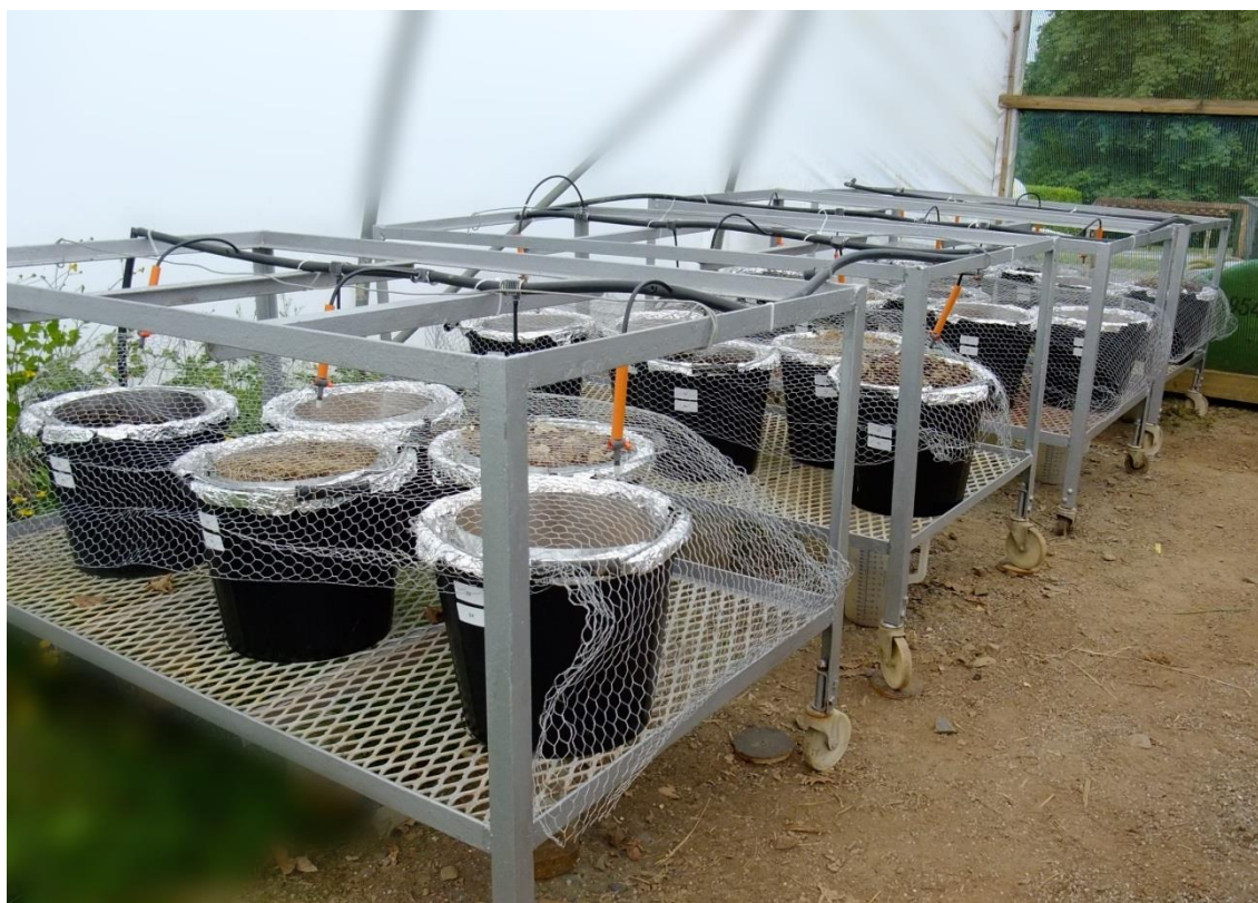
Figure 4.1. Experiment setup showing lysimeters with decomposing plant litter on packed soil cores with an overhead irrigation system, and provision for leachate collection below the trolleys.
