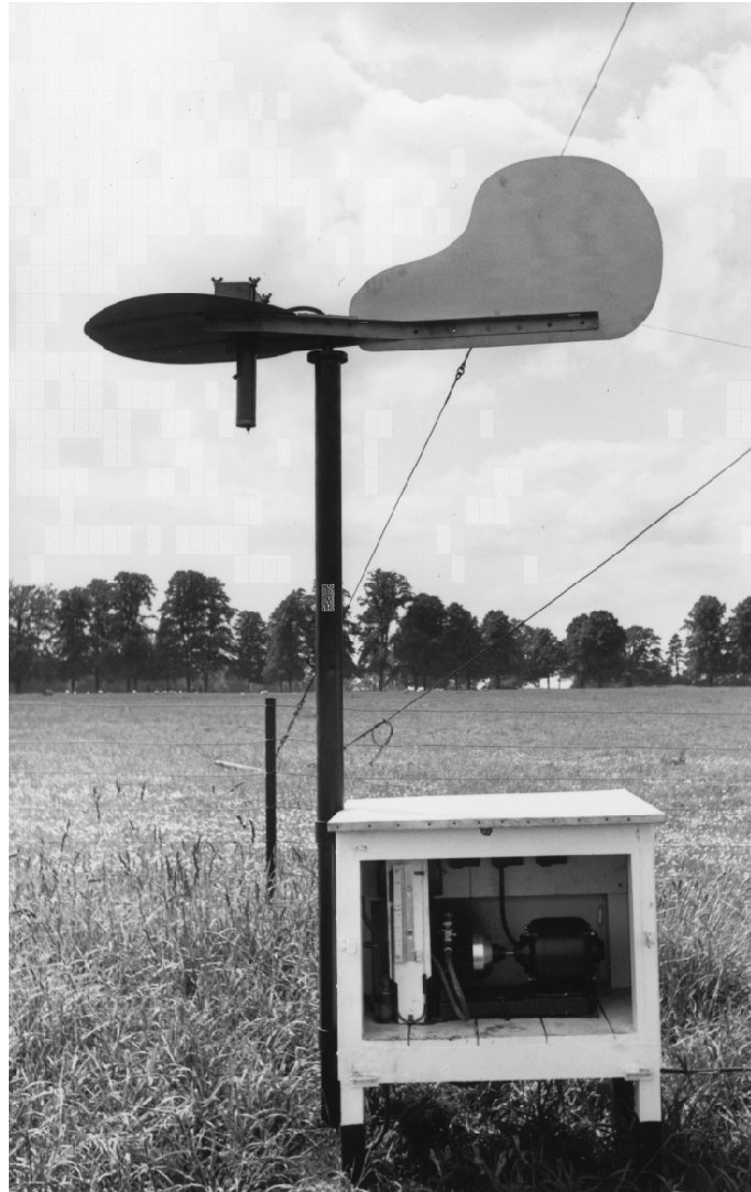
Figure 1. The Hirst spore trap: an early model. Photograph courtesy of IACR-Rothamsted.
