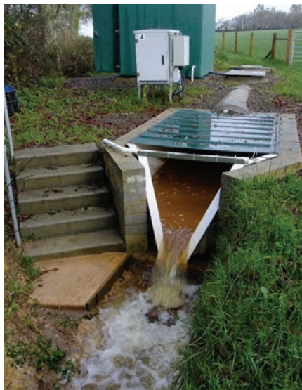
Catchment flumes and instrumentation cabin
