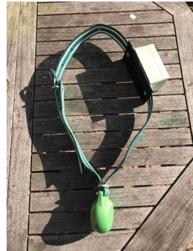
Figure 1. Neck collar and 'node' box for GPS transmission.
